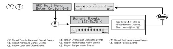
Open (Disarm) Report is sent with a CID **E409 C00?** Keyswitch / Close (Arm) Report is sent with a CID **R409 C00?** Keyswitch **Programming Setup for Texecom Premier 832 Keyswitch using a Zone**
