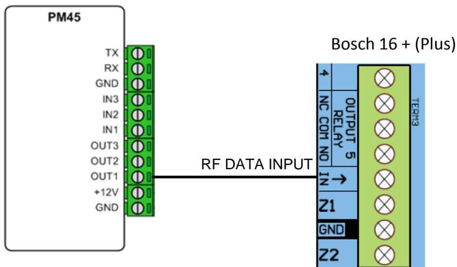
**E.g. 2:- Using a Zone:** Choose any hardwired zone 1-8, Zn Dbl 9-16 can be programmed as a keyswitch.
