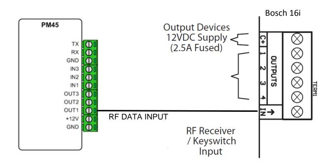
E.g. 2:- Using a Zone: Choose any hardwired zone 1-8, Zn Dbl 9-16 can be programmed as a keyswitch.
