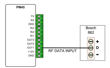
E.g. 2:- Using a Zone: Choose any hardwired zone 1-4, Zn Dbl 5-8 can be programmed as a keyswitch.
