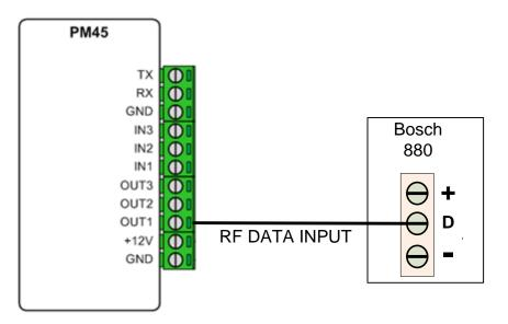
**E.g. 2:- Using a Zone:** Choose any hardwired zone 1-4, Zn Dbl 5-8 can be programmed as a keyswitch. NB: The other zone on the same terminals MUST be an Entry / Exit zone type.
