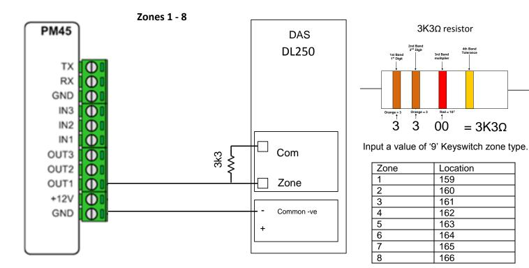
If the Opening / Closing communicator codes are enabled, Key Switch arming/ disarming will report via user code 14.
