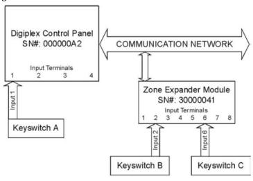
Keyswitch Zone # Section Serial# Input# Keyswitch A: 1 = [049] 000000A2 001 Keyswitch B: 2 = [050] 30000041 002 Keyswitch C: 3 = [051] 30000041 006
