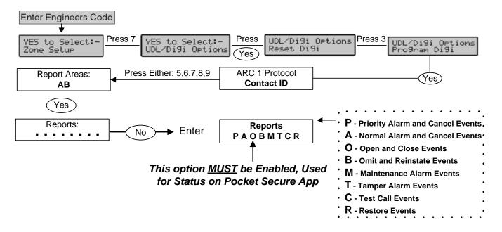
Open (Disarm) Report is sent with a CID **E409 C00?** Keyswitch / Close (Arm) Report is sent with a CID **R409 C00?** Keyswitch Programming a Keyswitch on a Texecom Premier 412 using a Zone.
