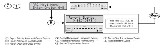
Open (Disarm) Report is sent with a CID **E409 C00?** Keyswitch / Close (Arm) Report is sent with a CID **R409 C00?** Keyswitch Programming a Keyswitch on a Texecom Premier 412 using a Zone
