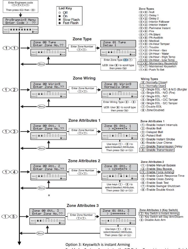
Enabled = System Arms instantly, NO Delay, Report is sent immediately. Disabled = Exit delay, Report is sent after Exit Delay
