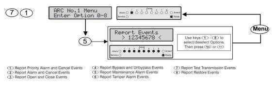
Open (Disarm) Report is sent with a CID E409 C00? Keyswitch / Close (Arm) Report is sent with a CID R409 C00? Keyswitch Programming a Keyswitch on a Texecom Premier 816 using a Zone
